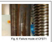
In all the other columns which the wrapping is done by layered it was observed that the origin point of the buckling was the un-bonded area. When the columns confined with GFRP strips (CFST1-L-a and CFST2-L-a), the zone confined with GFRP strips become more rigid due to the greater confinement pressure exerted by the GFRP strips. As a result the buckling of steel tube occurred without any rupture of fibre.
